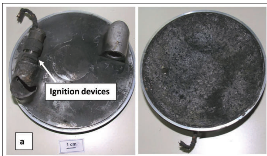
Figure 1. The Failed Booster Head End of the Pyro Housing (PH-1) (a) Front and (b) Back in the As-received Condition.
