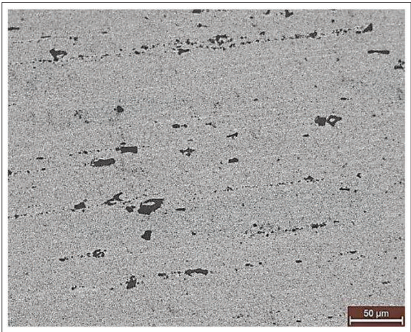
Figure 8. The Optical Microstructures Prepared from Heat-affected Zones of PH-2.
