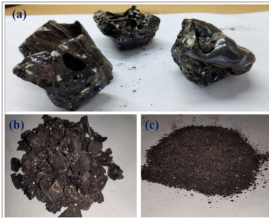
Figure 2. (a) untreated cupola slag, (b) cupola slag prepared as coarse aggregate and (c) cupola slag prepared as fine aggregate.
