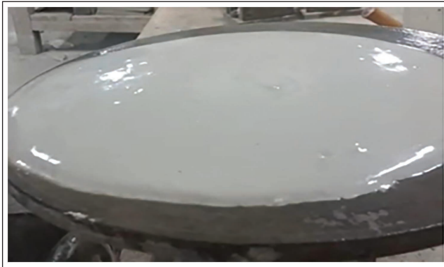
Figure 4. Flow Table Test of Cupola Slag-Based Cement.
